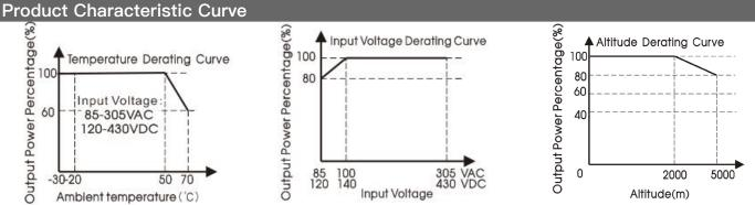
Note: 1) With an input voltage between 85-100VAC and a DC input between 120-140VDC the output power must be derated as per the temperature derating curves;
